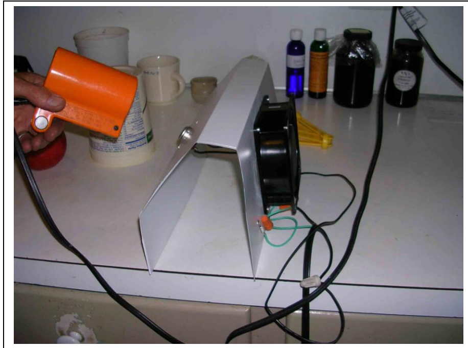
Above: Picture 3. Testing thermostat and fan in shroud assembly prior to installation
