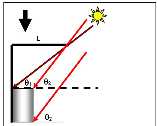
These angles are, respectively, 39.2 degrees and 53.7 degrees. What this means is that when the sun's angle above the horizon is equal to or less than these values, the barrels will, respectively, receive full solar illumination or receive illumination fully on their front
